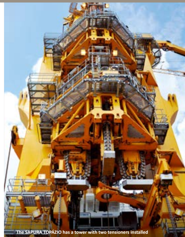
The traction winch of the SAPURA TOPAZIO
