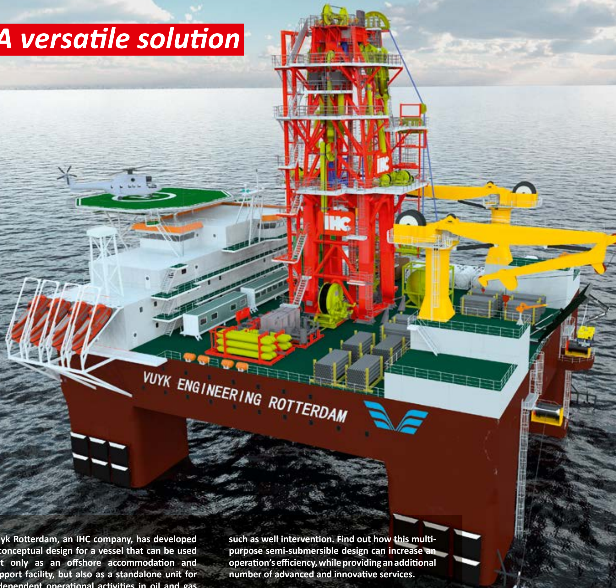
1. Semi-submersible vessel equipped with well intervention tower
